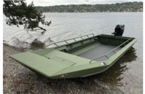
Wooldridge Boats exclusive jet tunnel offers the best in shallow water running and handling in challenging river running conditions. The tunnel allows the jet foot to be raised for protection, a clean water feed and ram effect. It also provides traction for controlled and predictable performance in tight quarters.
