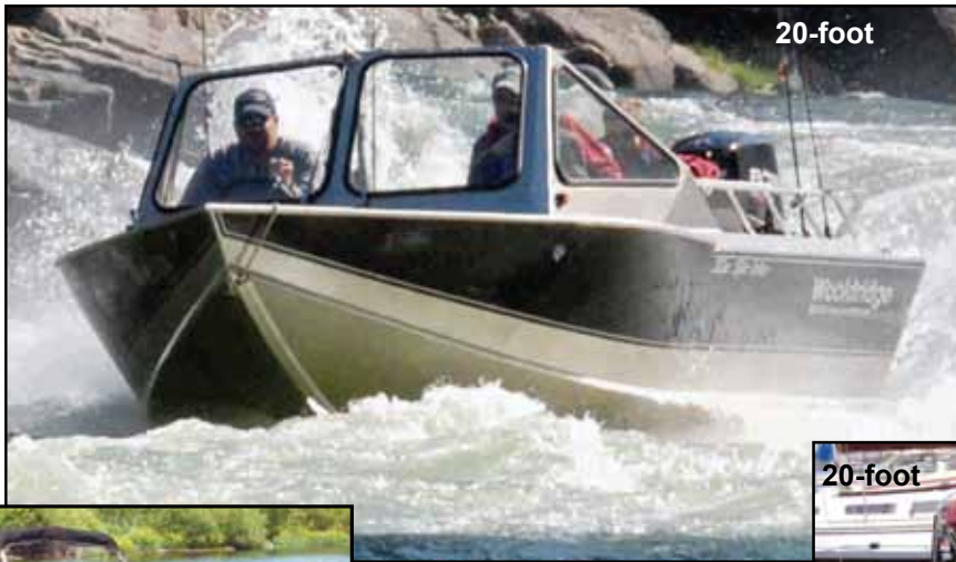
Wooldridge SS Drifter Outboard serves sportsmen in lengths of 20', 23' and 25', sedan or open boat (console or tiller). Wide bottom, high sides and exclusive Wooldridge jet tunnel are standard.
